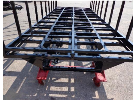
Fully Welded Frame / 24" centers
