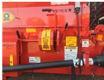
Removable Roof / 3-18" drum augers / simple controls Marine Treated Floor / 667H pintle aprons – all standard
