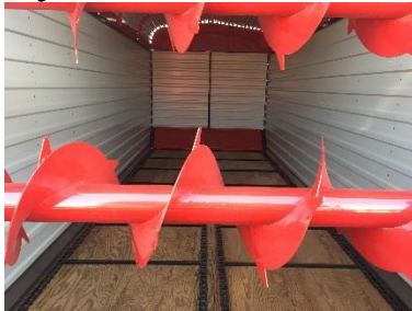
Removable Roof / 3-18" drum augers / simple controls Marine Treated Floor / 667H pintle aprons – all standard
